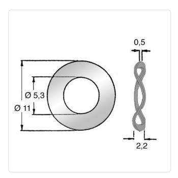
DIN/ISO: DIN137B Finish: Plain For Thread Size: M5 0.5 Height [mm]: Inner Diameter [mm]: 5.3
