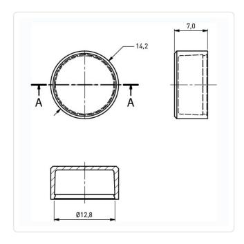
Color: Black Head Height [mm]: 7 Inner Diameter [mm]: 12.8 Material: PA 6 Material Group: Kunststoff
