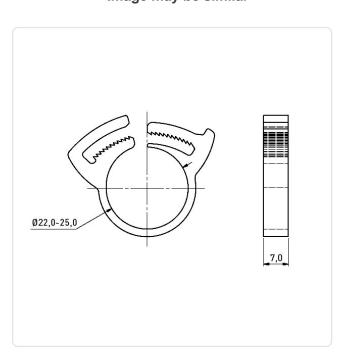
Color: Black Flammability Class: UL94-V2 PA 6.6 Material: Panel Thickness Range [mm]: 22,0-25,0
