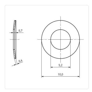
DIN/ISO: **DIN2093** Finish: Plain For Thread Size: M5 0.4 Height [mm]: Inner Diameter [mm]: 5.2
