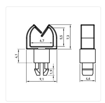
Bundle Diameter [mm]: 3,0-6,5 Color: Natural Height [mm]: 4.1 PA 6.6 Material: Mounting Hole [mm]: 3.8 Panel Thickness [mm]: 1,6 mm Width [mm]: 9.1 Weight: 0.23g
