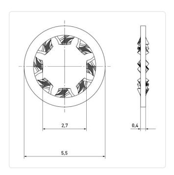
DIN/ISO: DIN6798I Finish: Plain For Thread Size: M2.5 0.4 Height [mm]:
