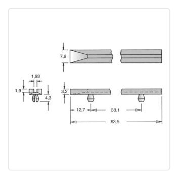
Color: Natural Dist. Mounting Holes [mm]: 38.1 Flammability Class: UL94-V2 Length [mm]: 63.5 Material: PA 6.6 Material Group: **Plastic** Model: Plug-In Foot
