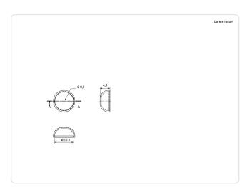
Color: Black Head Height [mm]: 4.3 Inner Diameter [mm]: 8.5 Material: PA 6 Material Group: **Plastic**
