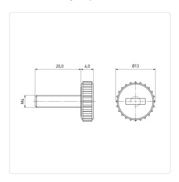
Color: Black Drive Type: Slotted Head Diameter [mm]: 13 Head Height [mm]:
