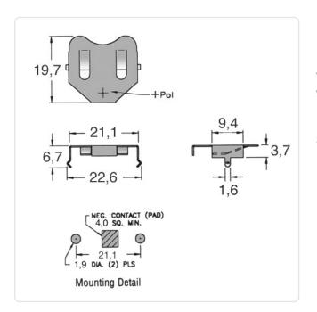
Battery Type: Cell Dia. 20mm
