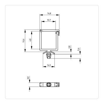
Bundle Diameter [mm]: 10,0-18,0 Color: Natural Height [mm]: 10.6 Material: PA 6.6 Model: Folding Mounting Hole [mm]: 4.8
