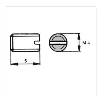
Color: Natural DIN/ISO: ISO4766 Drive Type: Slotted Flammability Class: UL94-V2
