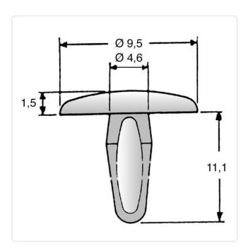
Color: Natural Flammability Class: UL94-V2 Head Diameter [mm]: 9.5 Material: PA 6.6 Material Group: **Plastic**
