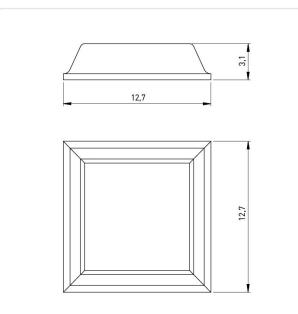
Bumper Design: Square, Tapered Color: Gray Diameter [mm]: 12.7 Flammability Class: UL94-HB Height [mm]: 3.1 Material: PUR - Polyurethane Weight: 0.55g Conformities: Reach RoHS **SVHC**
