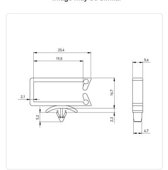
Bundle Diameter [mm]: 10,0-25,0 Natural Color: Height [mm]: 16.7 Material: PA 6.6 Mounting Hole [mm]: 4.8 Width [mm]: 25.5 Weight: 1.15g
