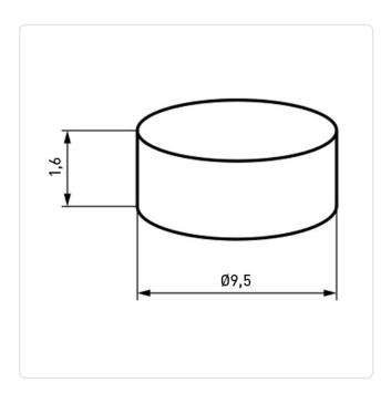
Bumper Design: Round Color: White Diameter [mm]: 9.5 Height [mm]: 1.6
