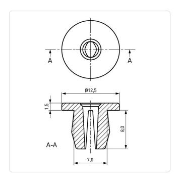
AF / OD [mm]: 12.5 Color: Natural Head Height [mm]: 1.5 Length [mm]: 8 PA 6.6 Material: Material Group: Plastic Panel Cutout [mm]: 7.0x7.0 Panel Thickness [mm]: 0,8-4,0 Thread Diameter [mm]: Ø 4.2 Weight: 0.47g Conformities:
