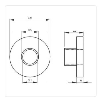
Color: Black Flammability Class: UL94-V0 Height [mm]: 2.2 Inner Diameter [mm]: 3.1 Lug Diameter [mm]: 3.5
