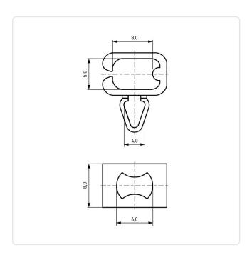
Bundle Diameter [mm]: 5,0-10,0 Color: Black Material: POM Mounting Hole [mm]: 5 Width [mm]: 8 Weight: 0.47g
